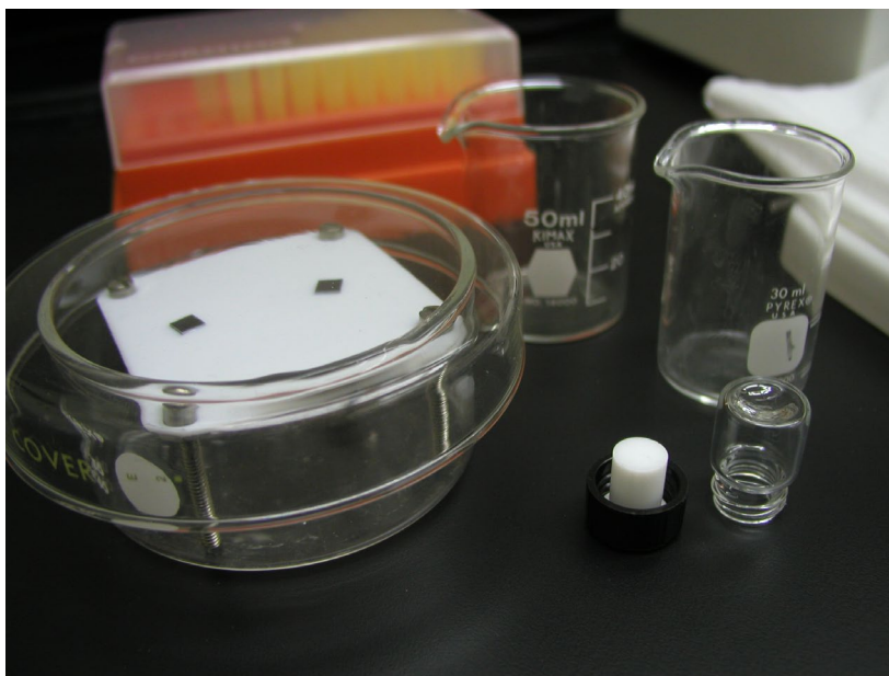
Figure 1. Apparatus used to functionalize and capture nanoparticles on TEM grids. Shown are the small glass vial with Teflon pedestal in the inverted cap, Teflon block with two test chips under cover, beakers used for dip rinsing, and a box of pipette tips.
